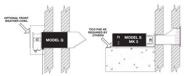
Model S units may be fitted vertically and ducted to an external wall, the fire/smoke damper must be fitted as close to the wall as possible
